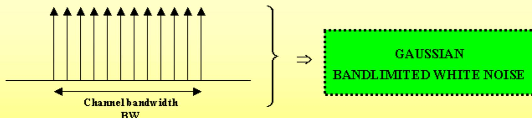
→ BASE BAND SIGNAL SYNTHESIS USING A COMPUTER CONTROLLED ARBITRARY WAVEFORM GENERATOR (AWG)
